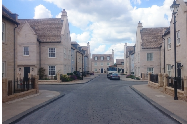
Figure 30: New street at Cecil Square, Stamford, uses traditional building forms, a limited palette of materials, interesting boundary treatments and a paved road surface to produce a distinctive street character.
