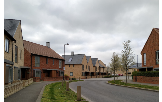
Figure 31: New street in Trumpington Meadows, Cambridge, combines many elements that define a strong street character, including non-standard highway treatments, quality contemporary materials, street trees, integrated sustainable drainage and windows on all building facades. The curve of the street leads the eye around the corner, creating further interest.
